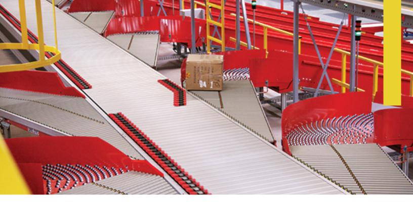
The VanRiet HC Sorter features a combination of high speed and narrow slats, which ensures one of the highest capacities in its class. Yet this does not come at the expense of the sorter's noise level. The application of low-noise and noise absorbing materials leads to the most silent sliding shoe sorter available on the market. This provides our customers a high sorting capacity, while retaining an ergonomic working environment.
